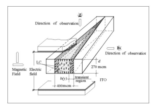
FIGURE: General scheme of the LC cell.
